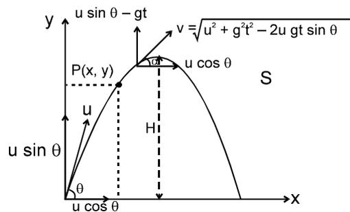
(i) Consider a projectile thrown with a velocity  $u$  making an angle  $\theta$  with the horizontal.
